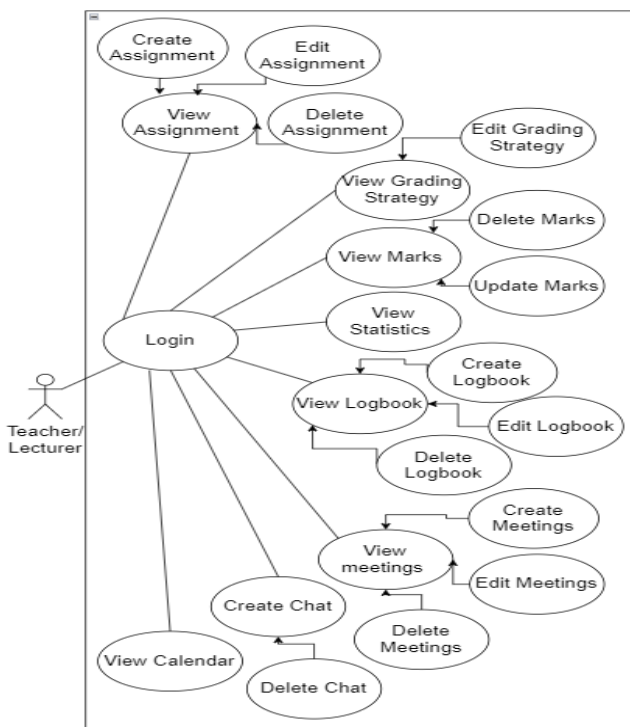
Fig. 6. Teachers' (primary and secondary school) and lecturer's use case diagram for proposed system
