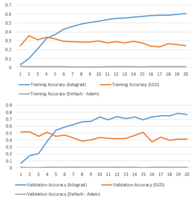
Fig. 6. (Results – Training and Validation Accuracy for different optimization functions of lr 0.1)
