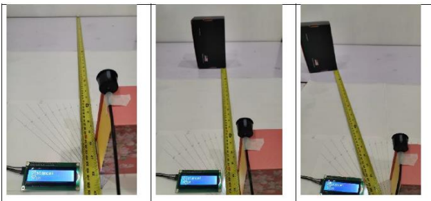
Fig. 12. Paper drawn with different angles using protractor
