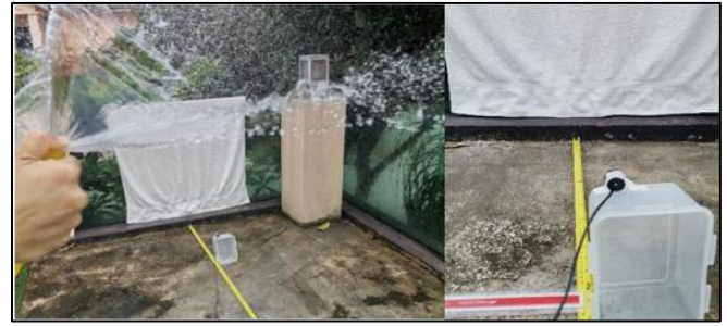
Fig. 10. set up of distance measurement test (Rain test)
