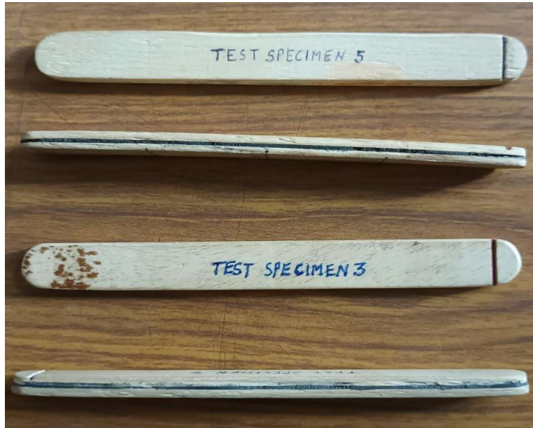
Fig 1. Composite Material developed using American Beech Wood and Epoxy Resin.
