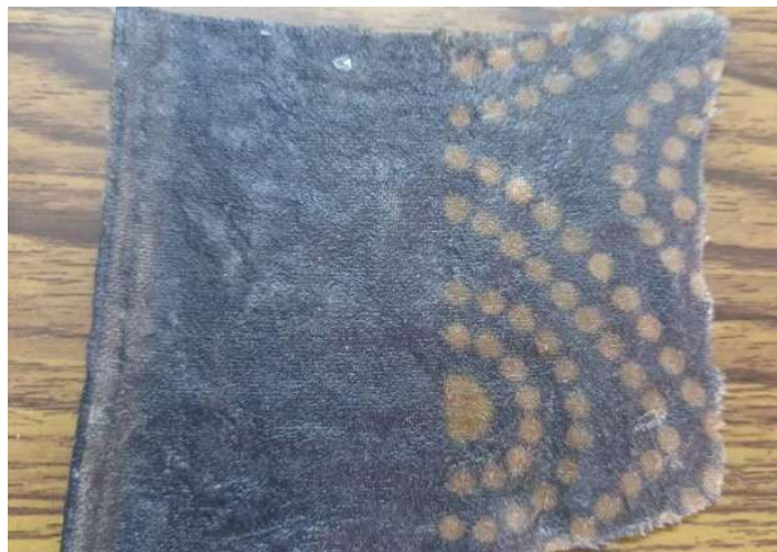
Fig 2. Cotton fiber soaked in Epoxy Resin with a considerable increase in strength.
