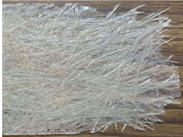
Fig 3. Fiber-Glass Epoxy Composite Panel developed by the author and students as a part of the “Teaching and Learning Process”.
