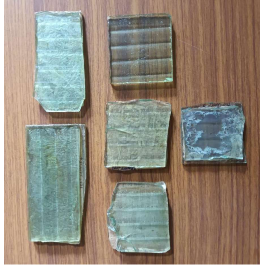
Fig 7. The glass-epoxy-soaked cotton fiber and glass-epoxy-soaked polypropylene composite for Panel Glass can provide resistance to glass getting split into a number of sharp parts when hit by an impact force.
